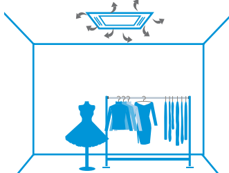
Air distribution with a dusty filter
